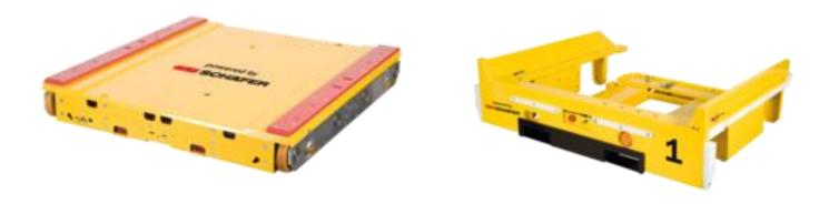
The operating principle: the docking station and the shuttle vehicle (orbiter) form a single unit that can be moved around the warehouse. Racks in which the shuttle operates have a centring console fitted onto the front.
