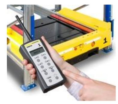
While the forklift attends to the next pallet to be stored, the orbiter transports the pallet quickly and safely to its desired storage location within the rack. Movement commands are given to the shuttle vehicle through a wireless remote control.
